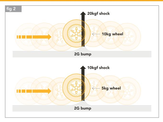
A high unsprung weight can also lead to "bouncing" and "hopping", where the tyres temporarily lose contact with an uneven road – which is potentially dangerous. You can significantly improve on this problem by installing Dymag's lightweight wheels – just look how much weight you could save!
