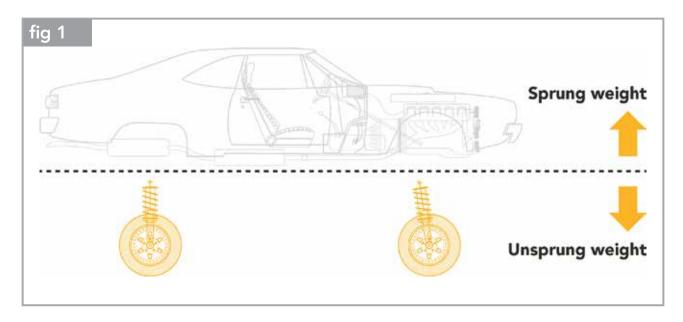
When a car passes over a bump in the road, the driver will feel the unsprung weight being forced upwards. At high speeds this causes unpleasant vibrations—the greater the vehicle's unsprung weight, the stronger these vibrations become.
