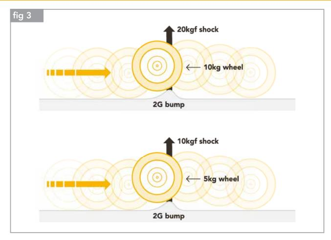
A high unsprung weight can also lead to "bouncing" and "hopping", where the tyres temporarily lose contact with an uneven road, causing the bike to buck around – which is potentially dangerous.
